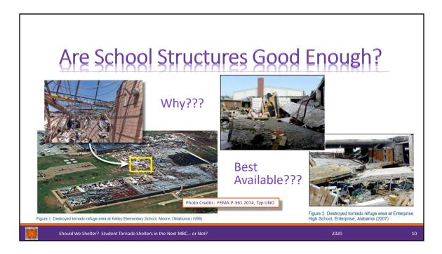
Why do we need specifically designed shelter spaces with well defined loads? History shows that areas previously thought to be 'safe' were not necessarily safe... The concept was good, but not sufficient to resist tornado wind loads, especially EF3 and greater....
